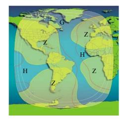
The footprints of the INTELSAT satellites are divided into various beams:
