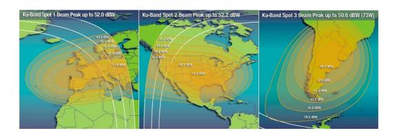
The global, hemispheric and zone beams use C-band frequencies. The spot beams use Ku-band frequencies.
