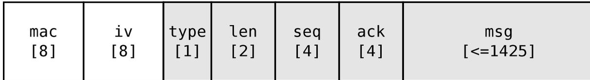
Figure 6.3: SkypeMorph UDP packet body layout, where the size (in bytes) is under the name for each field. The shaded parts are encrypted using 256-bit AES counter mode. All bytes after the mac field are included in the HMAC-SHA256-64 computation.
